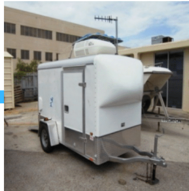
Left to right: a) HF-radar antenna (left) b) Mobile HF-radar unit (Center) & c) Inside of mobile unit (right) which contains the data acquisition and processing system along with other necessary components.
